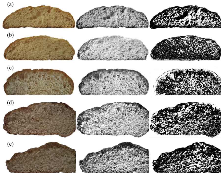
Fig. 2. Bread crumb structure at different new generation enzyme (NGE) concentrations: (a) B_0 , (b) B_{0.25} , (c) B_{0.50} , (d) B_{0.75} , and (e) B_{1.0} . The left panel corresponds to optical images, while in the center and right panel are images in grayscale and binarized.
